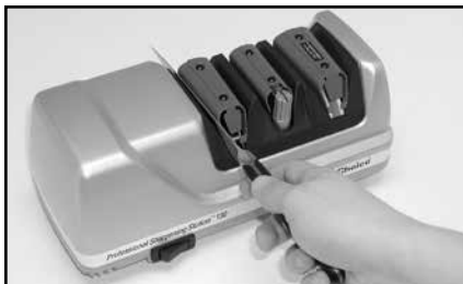
Figure 3. Stage 1. Inserting blade in slot between guide and elastomeric spring. Alternate individual pulls in right and left slots.
